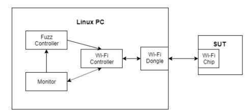
Figure 6.1: Fuzzing setup diagram
