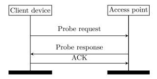
Figure 3.4: Active scanning sequence diagram
