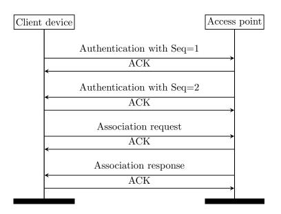
Figure 3.6: Authentication and association sequence diagram with an unprotected network
